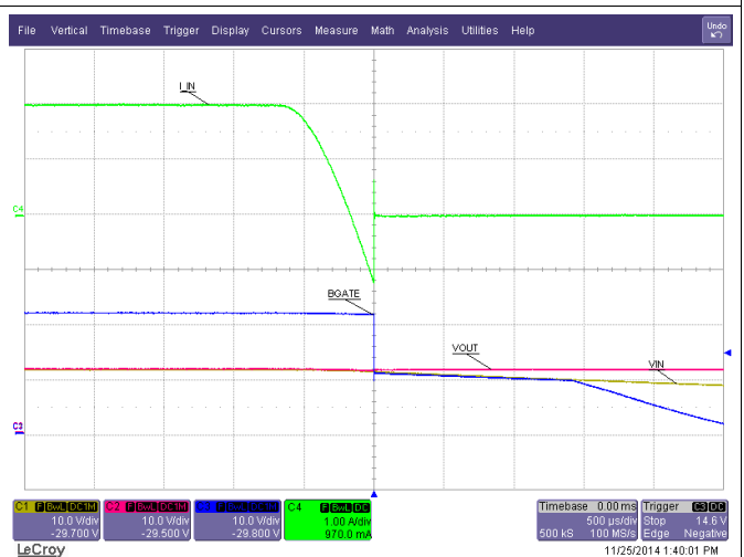
Figure 53. Gradual Reverse Current
