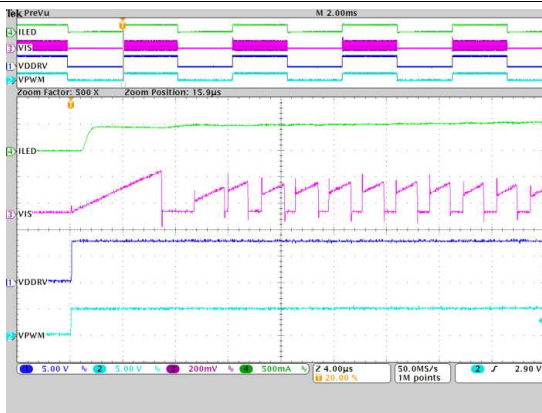
Ch1: DDRV voltage; Ch2: PWM input; Ch3: Switch sense current resistor voltage; Ch4: LED current; Time: 4 \mu s/div Figure 39. PWM Dimming Transient (Zoomed)
