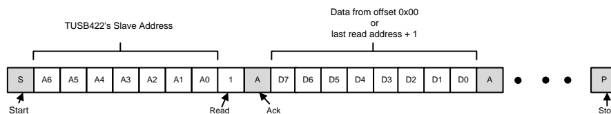
Figure 7. I2C Read Without Repeated Start
