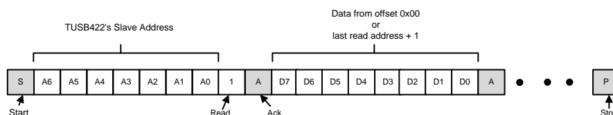
图 7. I2C Read Without Repeated Start
