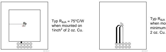
Typ  $R_{\theta JA} = 230^{\circ}C/W$ when mounted on minimum pad area of 2 oz. Cu.
