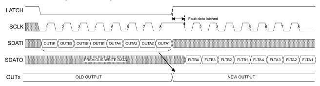
Figure 9. Daisy-Chain Serial Transaction
