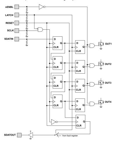
Figure 6. Serial Interface Operation
