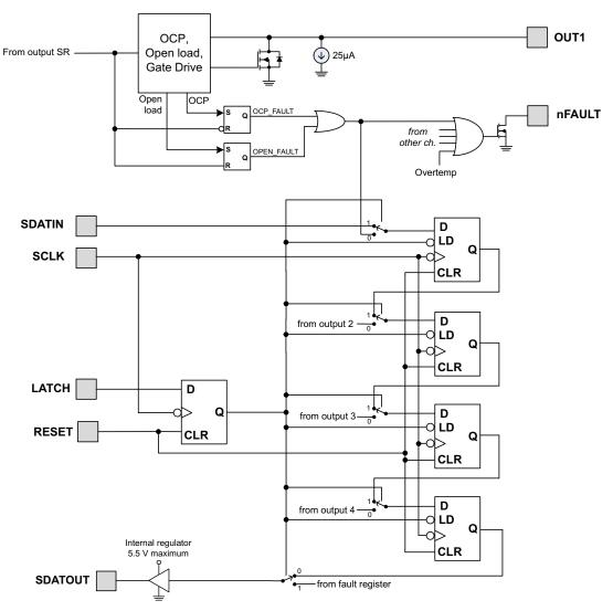
Figure 7. Fault Output
