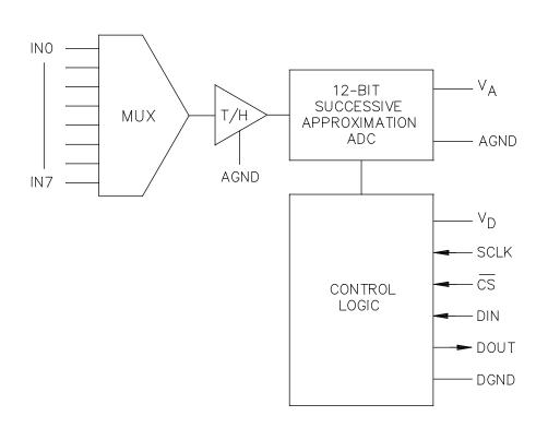
FIGURE 2. Block diagram.
