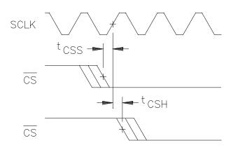
SCLK AND CS TIMING WAVEFORMS
