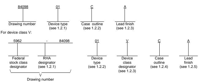
1.2.1 <u>RHA designator</u>. Device classes Q and V RHA marked devices meet the MIL-PRF-38535 specified RHA levels and are marked with the appropriate RHA designator. Device class M RHA marked devices meet the MIL-PRF-38535, appendix A specified RHA levels and are marked with the appropriate RHA designator. A dash (-) indicates a non-RHA device.
