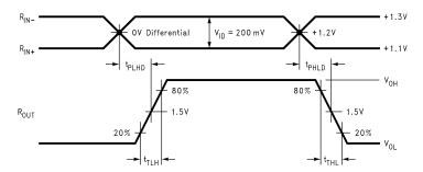
Figure 5. Receiver Propagation Delay and Transition Time Waveforms
