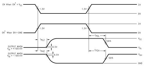
Figure 7. Receiver TRI-STATE Delay Waveforms
