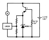
\*2N3638 or 2N2907 select for inverse  $H_{FE} \approx 5$ †Select for operation at 1.3V  $\ddagger I_Q \approx 600 \mu A$  to 900 $\mu A$
