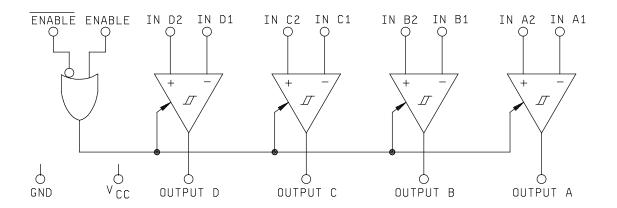
FIGURE 4. Logic diagram.
