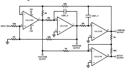
Figure 25. Universal State Variable Filter
