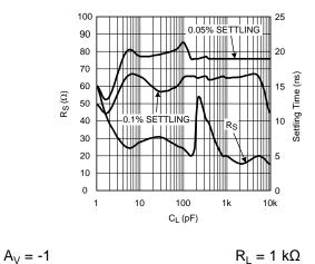
Figure 27. R<sub>S</sub> and Settling Time vs C<sub>L</sub>
