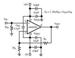
Figure 24. Recommended Non-Inverting Gain Circuit
