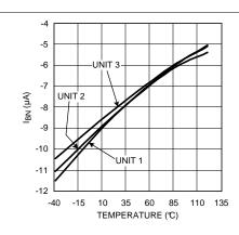
Figure 15. Inverting Input Bias for 3 Representative Units
