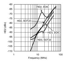
Figure 23. SOIC and SOT-23 Packages Distortion Terms Compared
