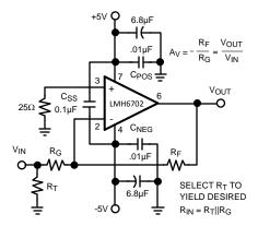
Figure 25. Recommended Inverting Gain Circuit
