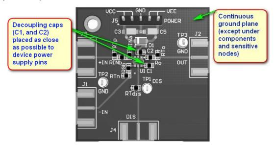
Figure 28. LMH6702 Evaluation Board Layer 1
