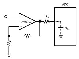
Figure 26. Input Amplifier to ADC
