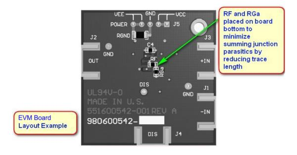
Figure 29. LMH6702 Evaluation Board Layer 2
