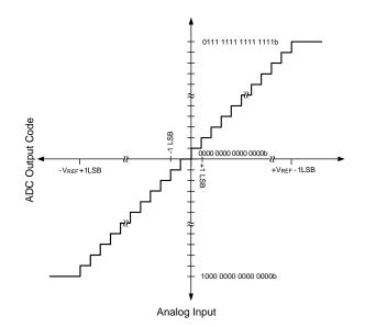
Figure 28. ADC Transfer Curve
