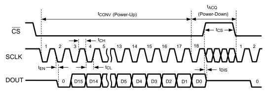
Figure 35. SM73201 Single Conversion Timing Diagram
