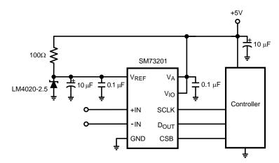
Figure 36. Low cost, low power Data Acquisition System
