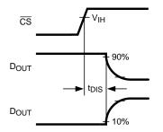
Figure 7. Voltage Waveform for t<sub>DIS</sub>
