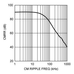
Figure 33. Analog Input CMRR vs. Frequency
