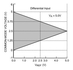
Figure 31.  $V_{CM}$  range for Differential Input operation
