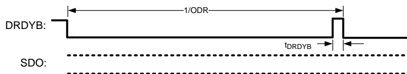
Figure 58. DRDYB Behavior for an ADC_DOUT not Read
