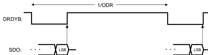
Figure 57. DRDYB Behavior for a Complete ADC_DOUT Reading
