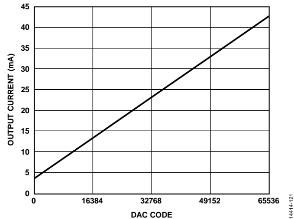
Figure 138. Gain Curve for ANA\_FULL\_SCALE\_CURRENT[9:0] = 1023 , DAC Offset = 3.8 mA
