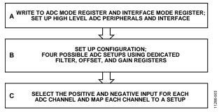
Figure 3. Configuration Flow
