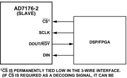
(IF CS IS REQUIRED AS A DECODING SIGNAL, IT CAN BE GENERATED FROM A PORT PIN.)
