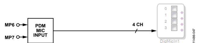
Figure 43. PDM Microphone Input Mapping to DSP in SigmaStudio
