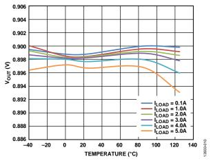
Figure 10. Output Voltage ( $V_{OUT}$ ) vs. Temperature,  $V_{OUT} = 0.9 V$
