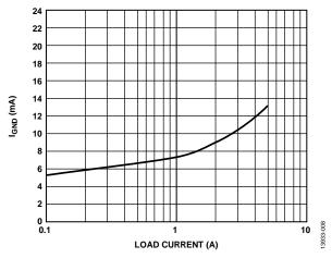
Figure 8. Ground Current ( $I_{GND}$ ) vs. Load Current ( $I_{LOAD}$ ),  $V_{OUT} = 1.3 V$
