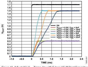
Figure 41. Adjustable V\_{OUT} Ramp-Up with External Soft Start Capacitor (V\_{OUT, EN}) vs. Time
