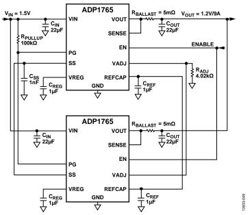
Figure 49. Two ADP1765 Devices Connected in Parallel to Achieve Higher Current Output
