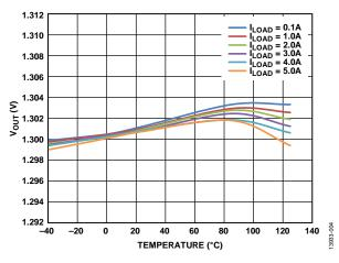
Figure 4. Output Voltage (Vout) vs. Temperature, Vout = 1.3 V
