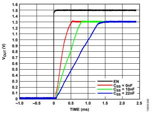
Figure 40. Fixed VOUT Ramp-Up with External Soft Start Capacitor (VOUT, EN) vs. Time
