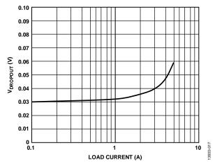
Figure 17. Dropout Voltage (V<sub>DROPOUT</sub>) vs. Load Current (I<sub>LOAD</sub>), V<sub>OUT</sub> = 1.3 V
