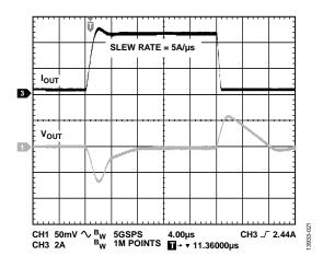
Figure 21. Load Transient Response,  $C_{OUT} = 47 \,\mu\text{F}$ ,  $V_{IN} = 1.8 \,\text{V}$ ,  $V_{OUT} = 1.3 \,\text{V}$
