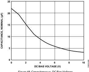
Figure 48. Capacitance vs. DC Bias Voltage
