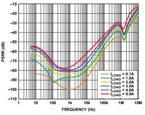
Figure 33. Power Supply Rejection Ratio (PSRR) vs. Frequency at Various Loads (I<sub>LOAD</sub>), V<sub>OUT</sub> = 1.3 V, V<sub>IN</sub> = 1.7 V
