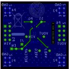
Figure 59. Typical Board Layout, Bottom Side
