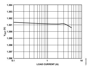
Figure 5. Output Voltage (Vout) vs. Load Current (ILOAD), Vout = 1.3 V
