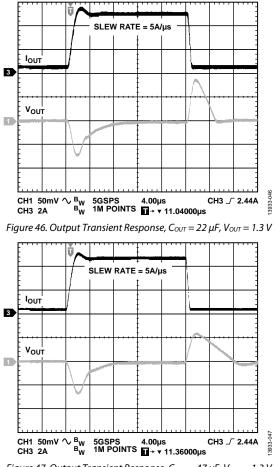
Figure 47. Output Transient Response,  $C_{OUT} = 47 \,\mu\text{F}$ ,  $V_{OUT} = 1.3 \,\text{V}$
