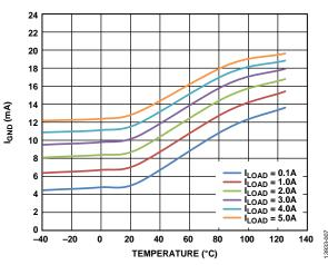
Figure 7. Ground Current ( $I_{GND}$ ) vs. Temperature,  $V_{OUT} = 1.3 V$
