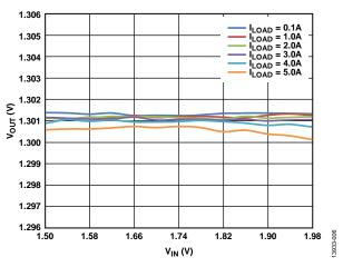
Figure 6. Output Voltage ( $V_{OUT}$ ) vs. Input Voltage ( $V_{IN}$ ),  $V_{OUT} = 1.3 V$
