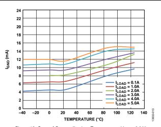
Figure 13. Ground Current ( $I_{GND}$ ) vs. Temperature,  $V_{OUT} = 0.9 V$
