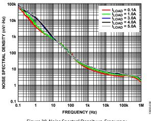
Figure 30. Noise Spectral Density vs. Frequency at Various Load Current (IOUT), 0.1 Hz to 1 MHz
