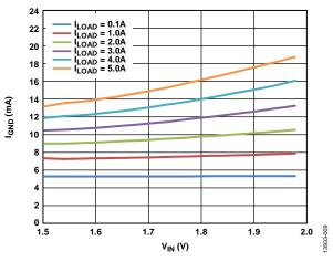
Figure 9. Ground Current ( $I_{GND}$ ) vs. Input Voltage ( $V_{IN}$ ),  $V_{OUT} = 1.3 V$
