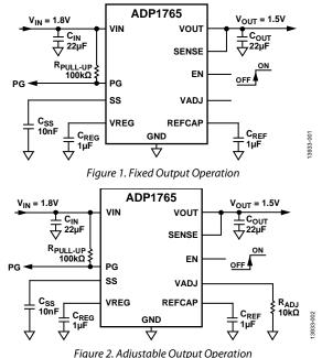
The ADP1765 is available in fixed output voltages ranging from 0.55 V to 1.5 V. The output voltage ( $V_{OUT}$ ) of the adjustable output model can be set from 0.5 V to 1.5 V through an external resistor connected between VADJ and ground.
