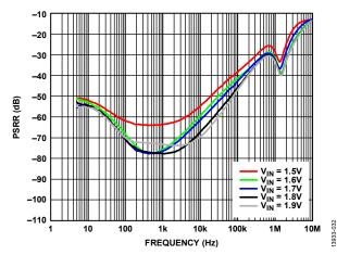
Figure 32. Power Supply Rejection Ratio (PSRR) vs. Frequency at Various Input Voltages (V<sub>IN</sub>), V<sub>OUT</sub> = 1.3 V, Load = 5 A
