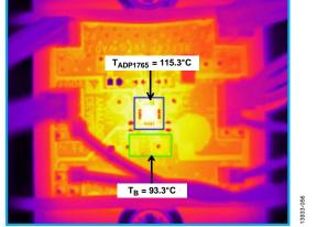
Figure 56. Thermal Image of the ADP1765 Evaluation Board at  $I_{LOAD} = 5$  A,  $V_{IN} = 1.5$  V,  $V_{OUT} = 1.3$  V,  $T_B = 93.3^{\circ}$ C
