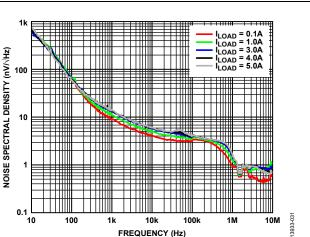
**FREQUENCY (Hz)** Figure 31. Noise Spectral Density vs. Frequency at Various Load Current (I<sub>OUT</sub>), 10 Hz to 10 MHz
