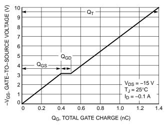
Figure 8. Gate-to-Source vs. Total Charge
