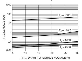
Figure 6. Drain-to-Source Leakage Current vs. Voltage
