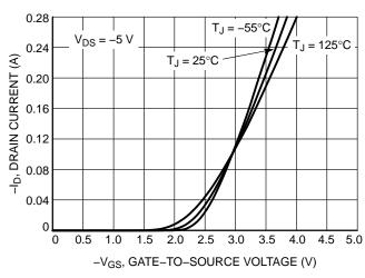
Figure 2. Transfer Characteristics
