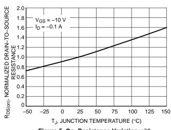
Figure 5. On-Resistance Variation with Temperature
