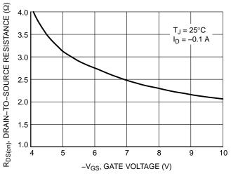
Figure 3. On-Resistance vs. Gate-to-Source Voltage
