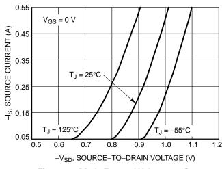
Figure 10. Diode Forward Voltage vs. Current
