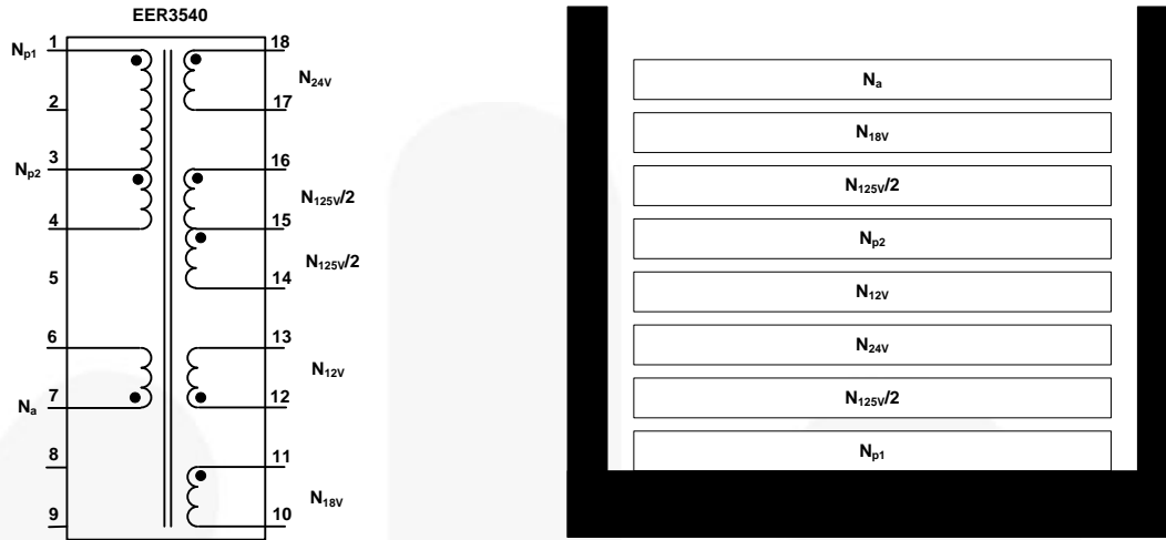
Figure 44. Transformer Schematic Diagram
