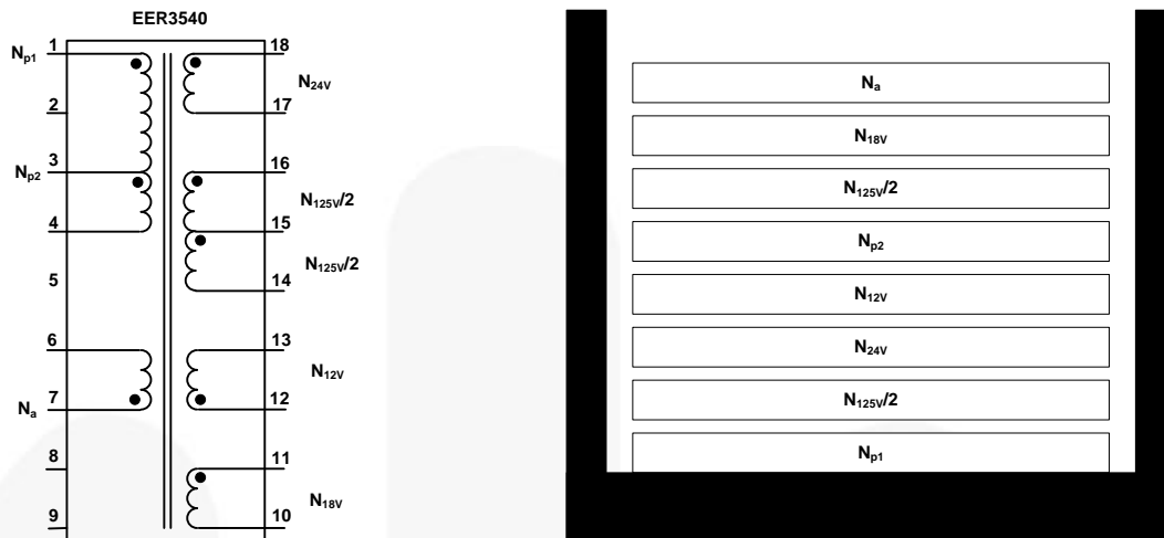
Figure 40. Transformer Schematic Diagram
