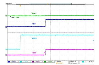
Figure 10. Auto-Charge Startup at VBUS Plug-in, OTG=0, V<sub>BAT</sub>=3.4 V
