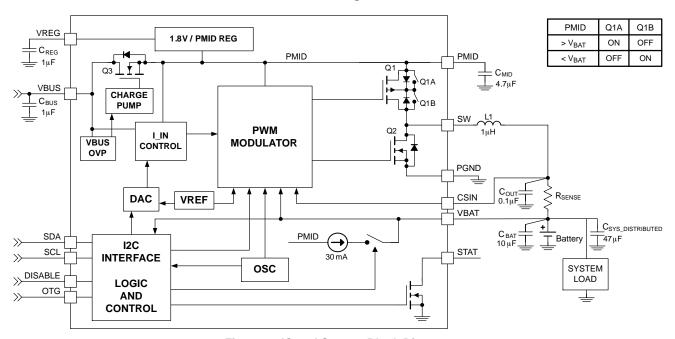
Figure 2. IC and System Block Diagram
