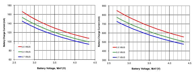
Figure 6. Battery Charge Current vs.  $V_{BUS}$  with  $I_{INLIM}$ =100 mA,  $V_{OREG}$ =4.35V
