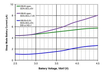
Figure 20. Battery Discharge Current vs. Mode
