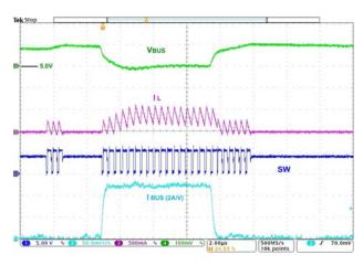
Figure 32. Load Transient, 5–155–5 mA, t<sub>R</sub>=t<sub>F</sub>=100 ns
