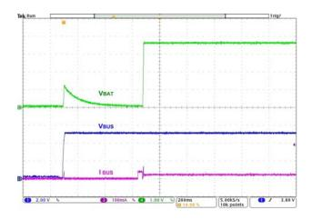
Figure 18. No Battery, TE=0, V<sub>BUS</sub> Power Up
