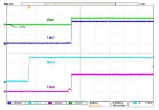
Figure 11. Auto-Charge Startup at VBUS Plug-in, OTG=1, V<sub>BAT</sub>=3.4 V
