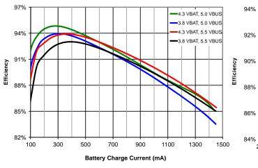
Figure 8. Charger Efficiency, No I<sub>INLIM</sub>,I<sub>OCHARGE</sub>=1450 mA
