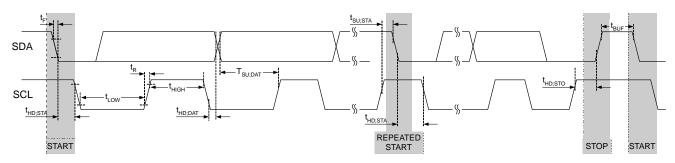
Figure 4. I<sup>2</sup>C Interface Timing for Fast and Slow Modes
