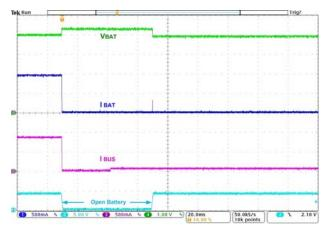
Figure 14. Battery Removal / Insertion During Charging,  $V_{BAT}$ =3.9 V,  $I_{OCHARGE}$ =1050 mA, No  $I_{INLIM}$ , TE=0
