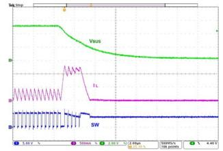
Figure 30. Startup, 3.6  $\text{V}_{\text{BAT}},$  44  $\Omega$  Load, Additional 10  $\mu\text{F},$  X5R Across  $\text{V}_{\text{BUS}}$
