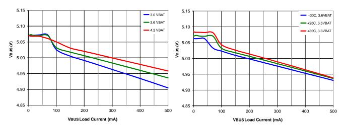
Figure 23. Output Regulation vs. V<sub>BAT</sub>
