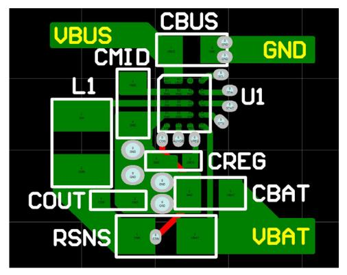
Figure 48. PCB Layout Recommendations
