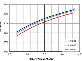
Figure 9. Charger Efficiency vs.  $V_{BUS}$ ,  $I_{INLIM}$ =500 mA,  $V_{OREG}$ =4.35
