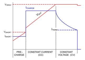
Figure 34. Charge Curve, I<sub>OCHARGE</sub> Not Limited by I<sub>INLIM</sub>
