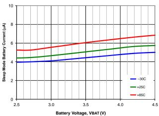
Figure 19. Sleep Mode Battery Discharge Current, SDA=SCL=0 V, VBUS Open
