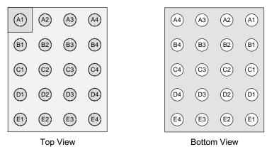
Figure 3. WLCSP-20 Pin Assignments
