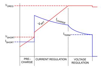
Figure 35. Charge Curve, I<sub>INLIM</sub> Limits I<sub>OCHARGE</sub>
