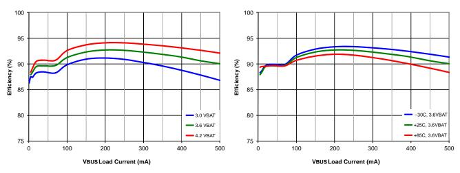
Figure 21. Efficiency vs. V<sub>BAT</sub>
