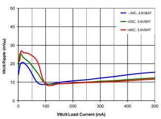
Figure 28. Output Ripple vs.  $V_{BAT}$
