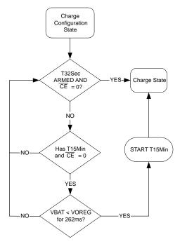
Figure 38. Charge Configuration
