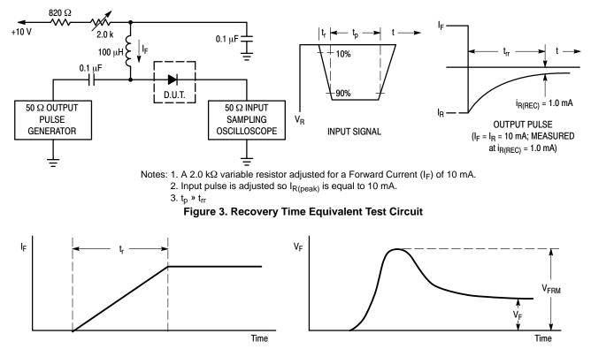
Figure 4. Peak Forward Recovery Voltage Definition
