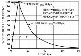
Figure 7. 8 x 20 µs Pulse Waveform
