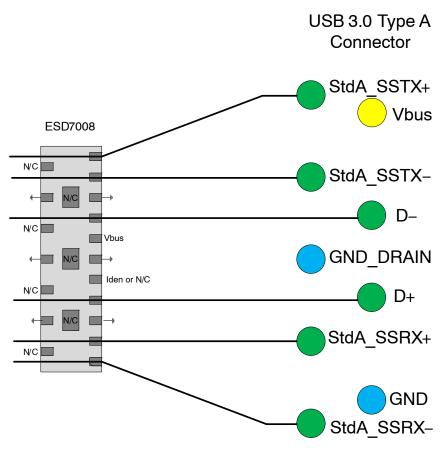
Figure 16. USB3.0 Layout Diagram
