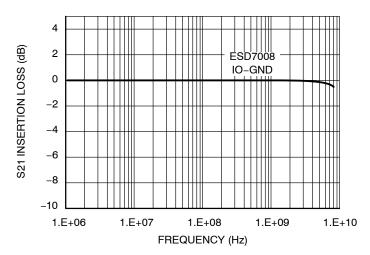
Figure 15. ESD7008 Insertion Loss
