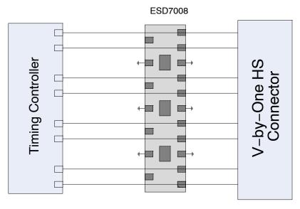
Figure 19. V-by-One HS Layout Diagram (for LCD Panel)
