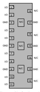
Figure 2. Pin Configuration
