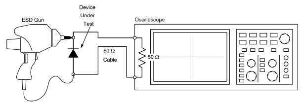
Figure 6. Diagram of ESD Clamping Voltage Test Setup
