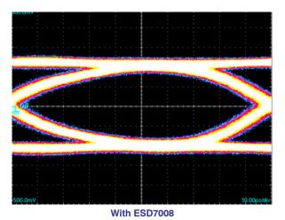
Figure 14. Thunderbolt Eye Diagram with and without ESD7008. 10 Gb/s, 400 mV<sub>PP</sub>
