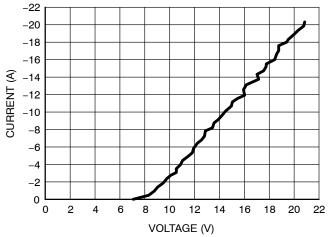
Figure 9. Negative TLP I-V Curve
