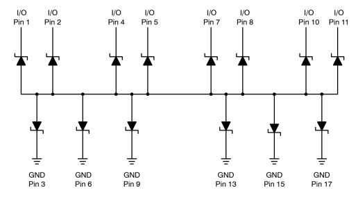
Note: Only Minimum of 1 GND connection required
