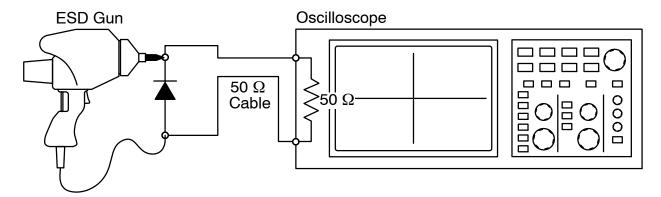
Figure 4. Diagram of ESD Test Setup
