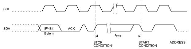
Figure 7. Write Cycle Timing
