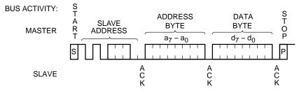
Figure 6. Byte Write Sequence
