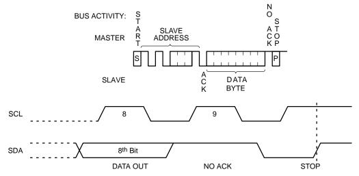
Figure 10. Immediate Read Sequence and Timing
