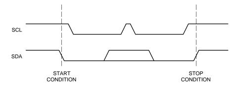
Figure 2. Start/Stop Timing
