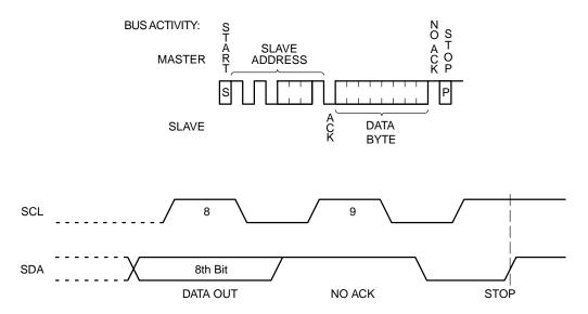
Figure 10. Immediate Read Sequence and Timing
