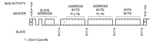
Figure 6. Byte Write Sequence
