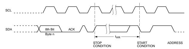
Figure 7. Write Cycle Timing
