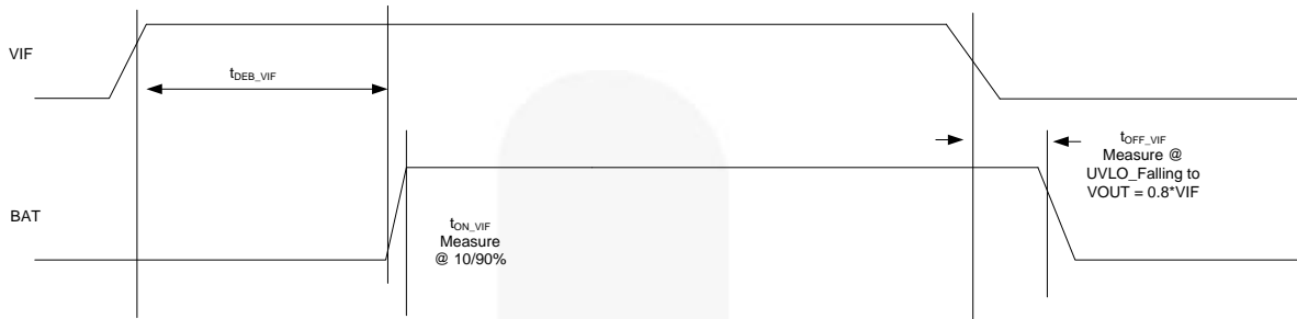
Figure 8. Timing for V_{IF} Power Up/Down and Normal Operation (ON=Don't Care)
