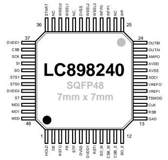
Figure 3: LC898240 Pinout
