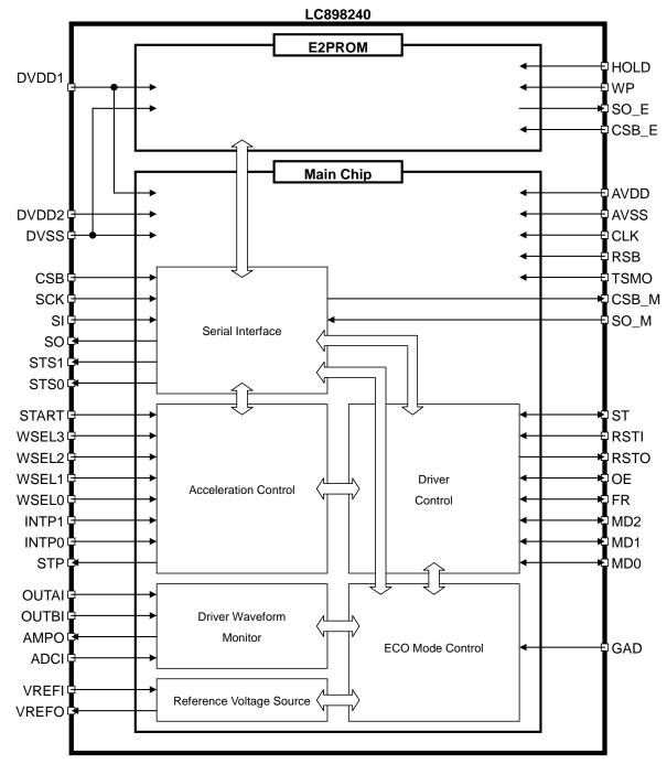
Figure 1 LC898240 Block Diagram
