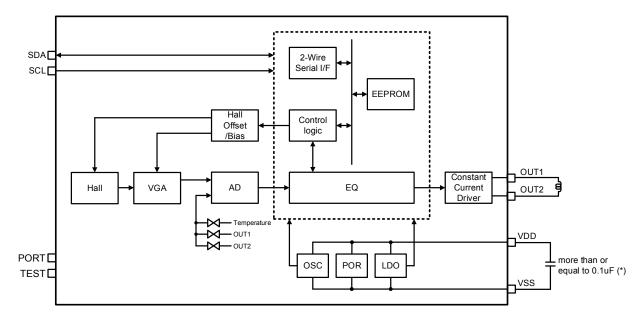
(\*): Consider capacitance of capacitor between  $V_{\mbox{DD}}$  and  $V_{\mbox{SS}}$ . According to power source environment, attach an additional capacitor in camera module.
