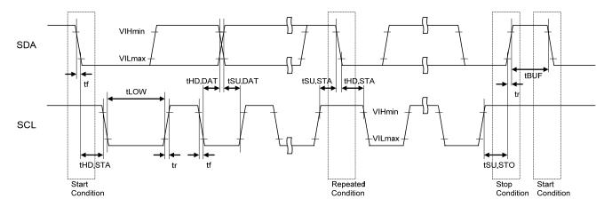
Figure. 2-wire serial interface timing definition
