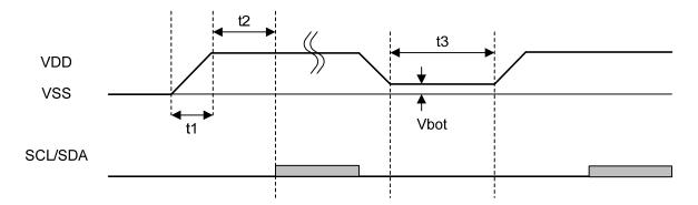
Figure. V<sub>DD</sub> supply timing
