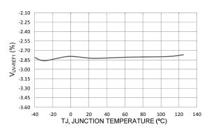
Figure 12 Vuv-REF1 vs. Temperature
