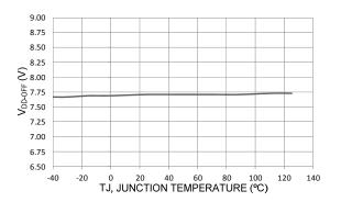
Figure 5 V<sub>DD-OFF</sub> vs. Temperature
