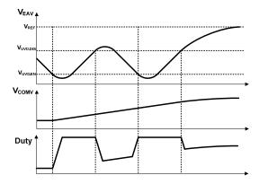
Figure 19. No to full load transient
