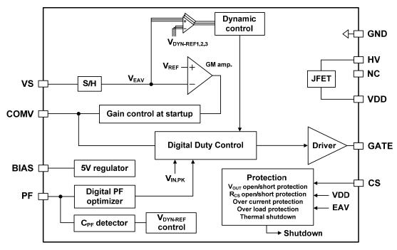
Figure 2. Simplified Block Diagram
