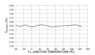
Figure 11 Vov-REF1 vs. Temperature
