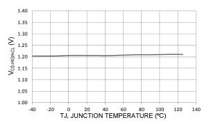
Figure 6 Vcs-High-cl vs. Temperature
