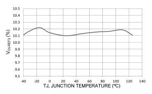
Figure 10 Vov-REF3 vs. Temperature
