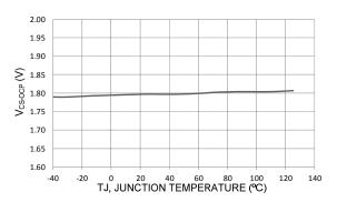
Figure 8 V<sub>CS-OCP</sub> vs. Temperature
