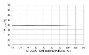
Figure 3 V<sub>DD-ON</sub> vs. Temperature
