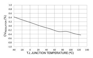
Figure 9 CVREGULATION vs. Temperature
