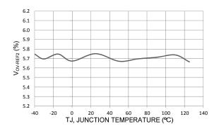
Figure 13  $V_{OV-REF2}$  vs. Temperature
