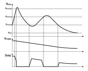
Figure 20. Full to no load transient
