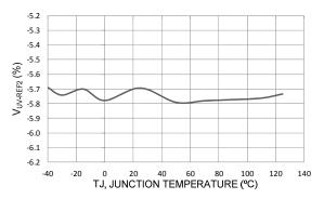
Figure 14  $V_{UV-REF2}$  vs. Temperature
