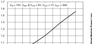
Figure 7. Power Loss vs. Output Current
