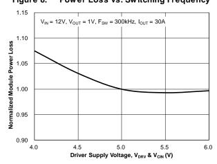
Figure 9. Power Loss vs. Input Voltage
