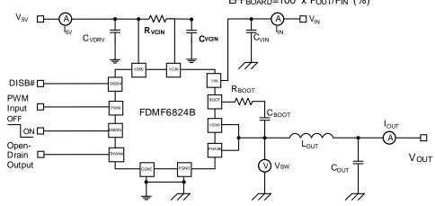
Figure 29. Block Diagram With V<sub>CIN</sub> Filter
