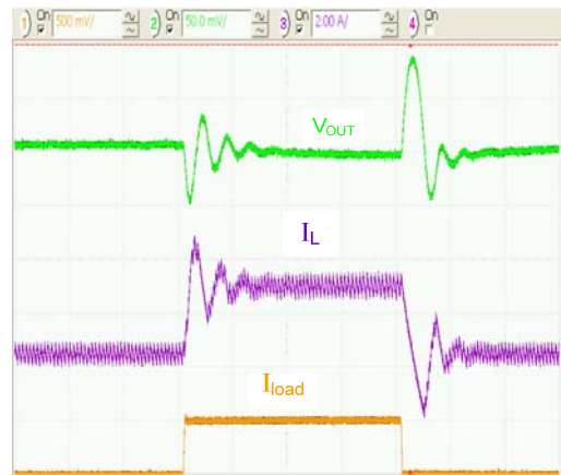
Figure 14. 500 mA to 3 A to 500 mA, 5 \mu\text{s}/\text{div} .
