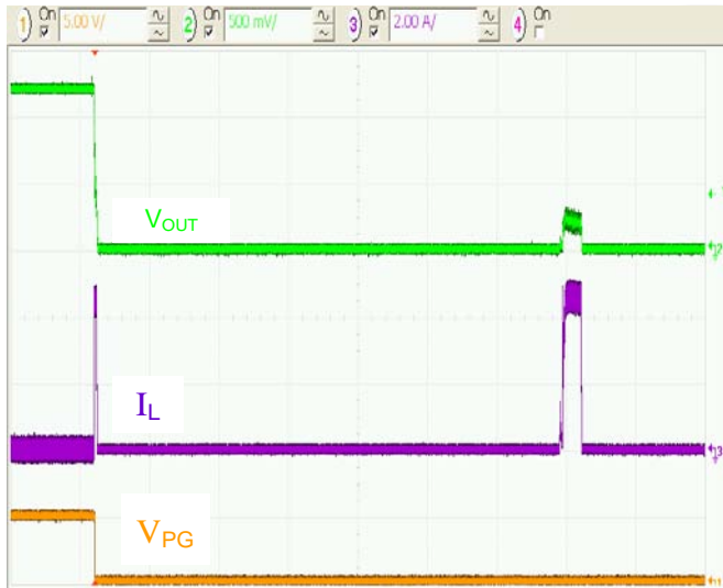
Figure 19. VOUT to GND Short Circuit, 200 \mu\text{s}/\text{div} .
