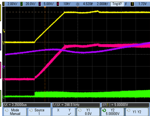
Figure 22. Start-Up Transition at 6A Load
