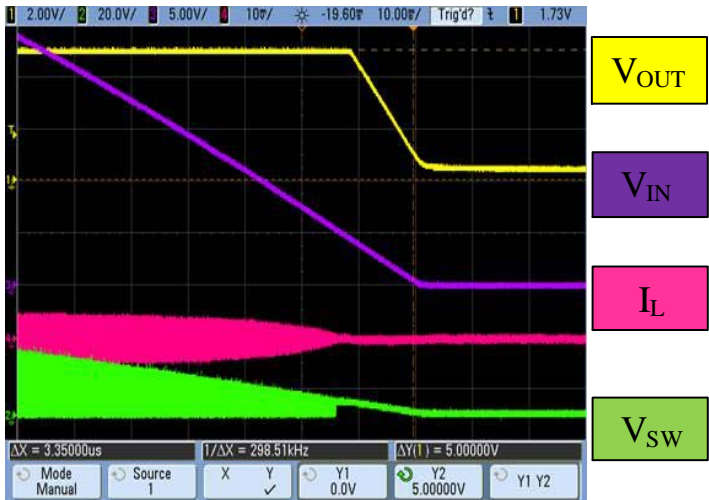
Figure 23. Shut-Down Transition at No Load
