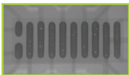
Figure 9: X-Ray of EPC2001 after solder stencil assembly process
