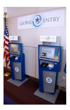
For users with visual impairment the EZ Access keypad often provides the most effective method of interaction with menu driven applications. This level of accessibility is not provided by the primarily visual interface offered by touch screens alone.
