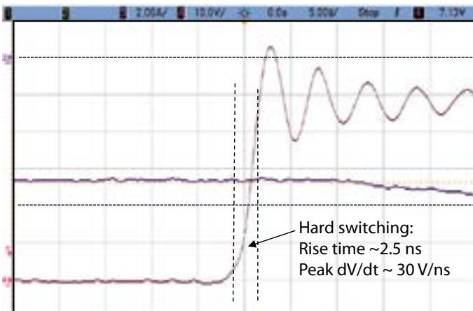
Figure 6: 48 V – 1.2 V eGaN FET hard switching transition time.
