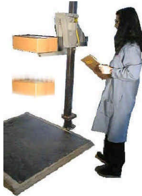
Drop testing simulates real-world conditions your products may face
