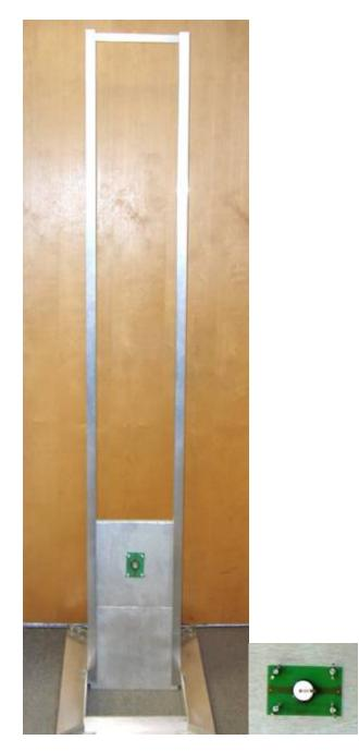
We used wing nuts for quick mounting of the same PCB to either the jarring or drop test fixtures.
