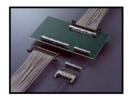
**The FI-E series** is a 1.0mm pitch board-to-wire connector series that supports LVDS with 14, 17, 30 position connectors. It features a mechanical lock to prevent incomplete or inadequate mating, a low profile design with 3.2mm height and durable guide alignment to permit blind mating. Cable options include discrete wires, fine-wire coaxial and FFC. *View FI-E datasheet for more information*.
