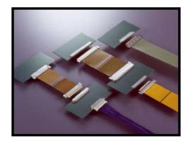
**The FI-X** series features a 1.0mm pitch slim line LVDS connector for high-density packaging. It offers a 1.0mm height off the board low-profile SMT type receptacle, available in 20 and 30 positions with locking features. Options include a crimp type cable plug for discrete wire, ZIF (Zero Insertion Force) type for FPC, and fine-wire coaxial type cables. *View FI-X datasheet for more information*.
