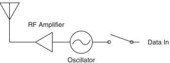
Figure 2: A Simple RF Transmitter
