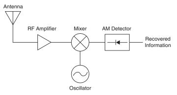
Figure 4: A Simple Superhet Receiver
