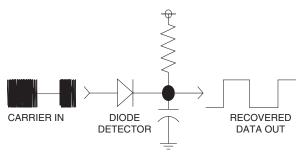
Figure 2: Diode Detector Circuit
