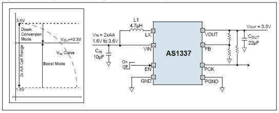
Figure 1. AS1337 - Typical Application Diagram - Dual Cell to 3.3V Synchronous Boost Converter
