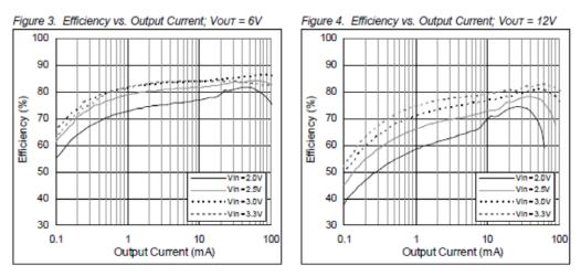
Fig. 3: Efficiency vs. Output Current for different Input Voltages of the AS1344
