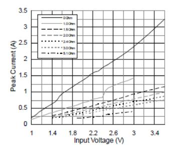
Fig. 2: Peak current vs. Input Voltage, for different values of external resistor
