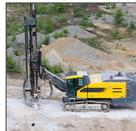
Drilling Machine (Mining)
