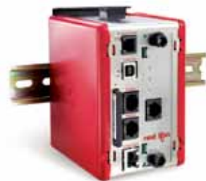
The Data Station Plus functions as both a data management platform and PFM host.
