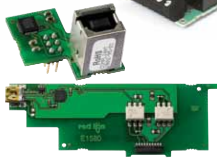
USB cards let you quickly connect to computers and communicate directly to the meters. No more messy converters.
