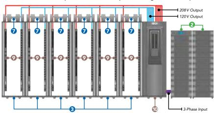
Centralized Backup Power (3-Phase Input and Single-Phase Output)
