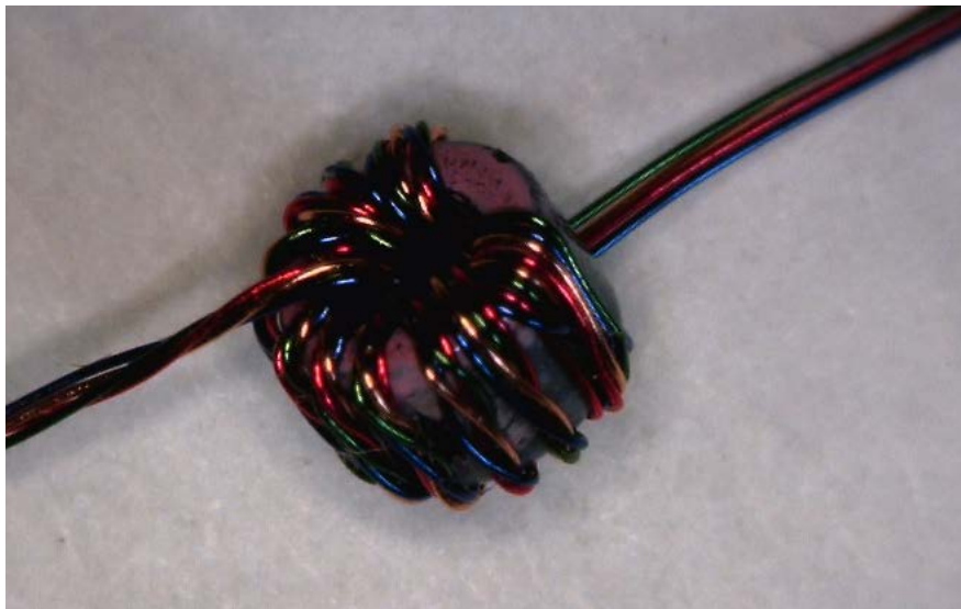
Figure 3. High Performance 10GbE LAN transformer utilizes twisted pairs
