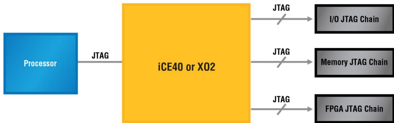
Fig. 3: JTAG Extender using a Lattice Semiconductor ULD FPGA.
